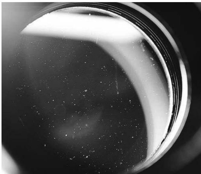
Fig. 2. Characteristic surface contamination of the optical system.
